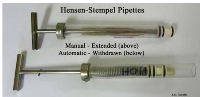
Figure 1. Hensen-Stempel pipettes are available in manual models (top) that must be pulled to obtain the sample or as spring-loaded models (bottom) that retract the sample automatically. The 1-ml size is typical, but larger styles are also available.
