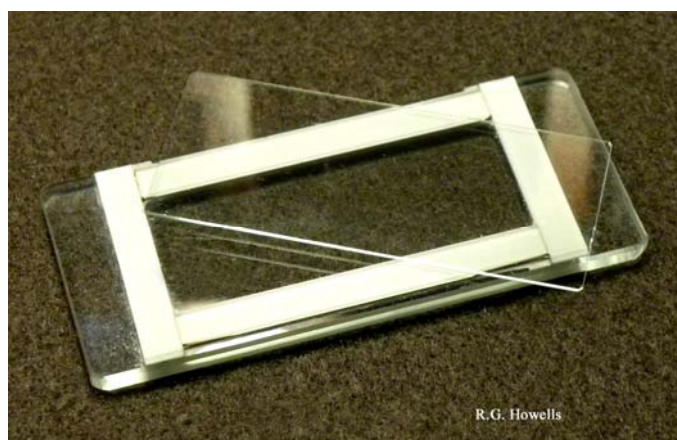
Figure 2. Sedgwick-Rafter cell used for counting plankton samples. This example holds 1 ml of sample.
